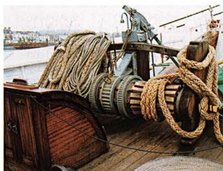
The windlass. With a lever inserted in the lefthand end too, one movement raises the anchor just 4in!
