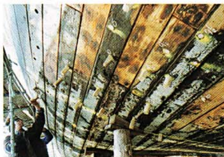
Knocking home the trenails.
