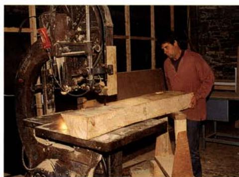
Far left: Kathleen & May looks out over Bideford's 'Ancient Bridge' and the waters of the Torridge Top left: sawing a new frame - when finished it will be 5" by 7" and will be used doubled at close spacing
